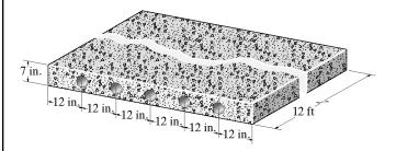
$$W = (144 \text{ lb/ft}^3)[(12 \text{ ft})(6 \text{ ft})(\frac{7}{12} \text{ ft}) - 5(12 \text{ ft})(\pi)(\frac{2}{12} \text{ ft})^2] = 5.29 \text{ k}$$
