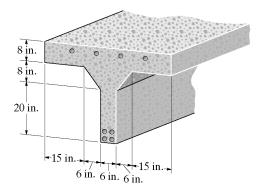
$$A = (28 \text{ in.})(6 \text{ in.}) + (8 \text{ in.})(48 \text{ in.}) + 2(\frac{1}{2})(6 \text{ in.})(8 \text{ in.}) = 600 \text{ in}^2 = 4.167 \text{ ft}^2$$
